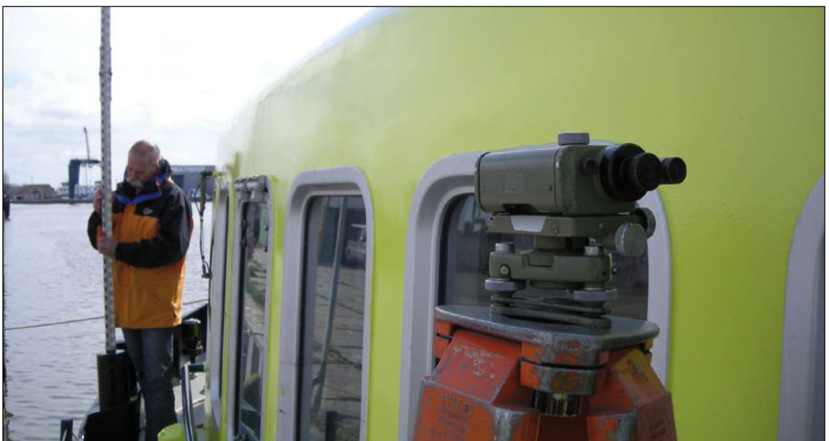
Figure 6: Pitch calibration onboard.
