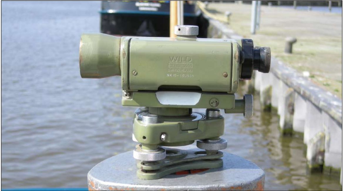
Figure 4: A tilting level set up for roll calibration.
